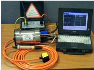
Figure 4 – ACFM topside equipment
