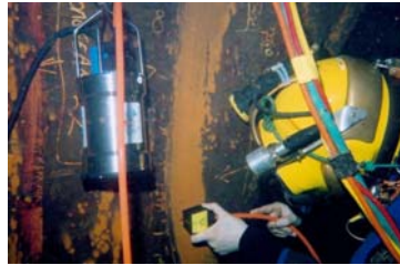
Figure 5 – ACFM subsea equipment
