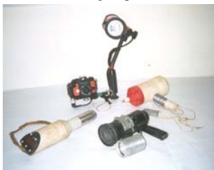
Figure 3 – Stills and video cameras, UT and CP meters
